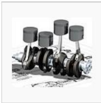
CAD drawing of crankshaft and pistons.
